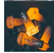
Forged components are widely used in machinery and equipment where high strength is required and usually undergo further processing to achieve their final shape. Forging produces parts stronger than those made by any other metal forming process."
